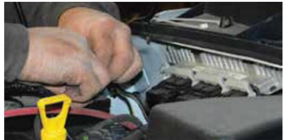
6. Install and connect the safety cut-off switch at any easy, reachable distance from the winch. We hooked the PS501R cable to the cut-off switch.
