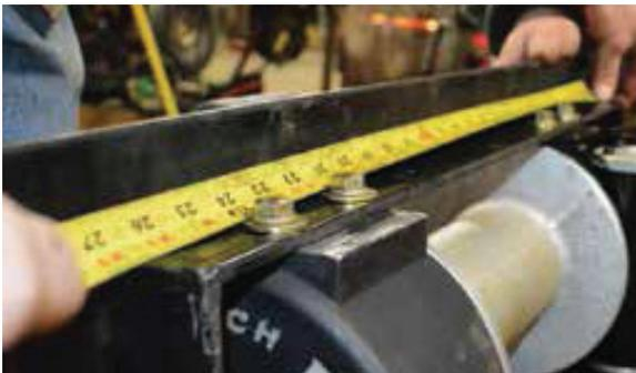
3. As dimensions match, place the winch carefully onto the truck bed. As shown, framing the angle mounts are an option for a clean, more finished look.
