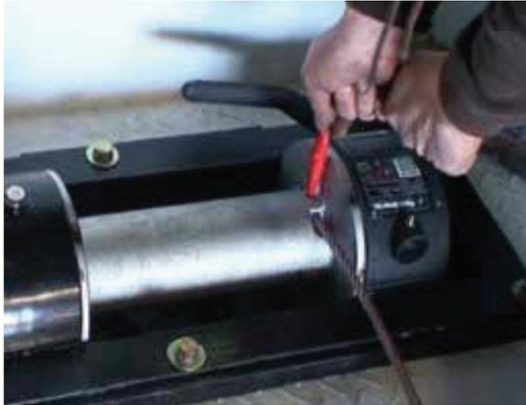
8. Next, power the newly mounted and installed winch. Pull the cable in while applying resistance and tension. Otherwise, the cable will let loose on you and will tangle on the drum.
