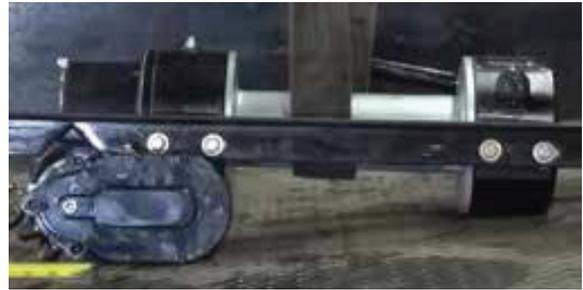
5. Next, connect the power cable from the solenoid to a positive power source. Wire a 4 gauge ground from the winch motor mounting bolt directly to the negative terminal of the truck battery using the PS501 or PS501X2.
