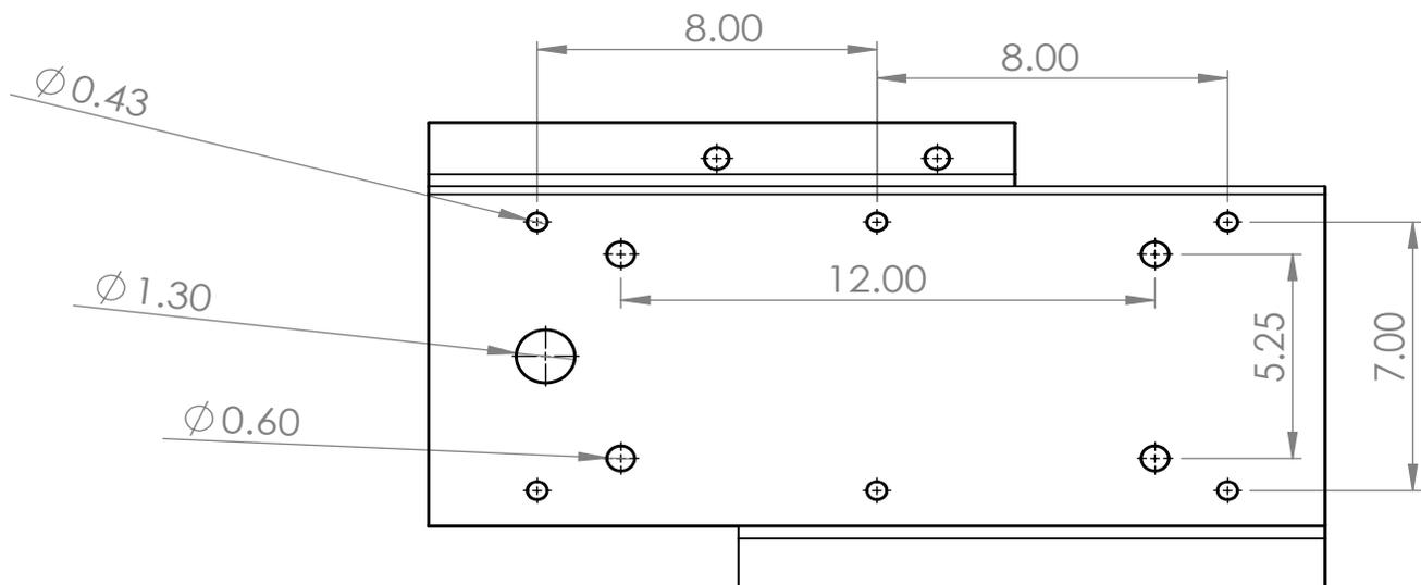
↑ *figure 3: Mounting pattern of the PBM1*
