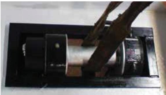
4. After successfully placing the winch on your truck, mount the frame. Using a total of eight grade 8, or "G8" bolts at least 3/8" thick is required. Lock washers as well.
