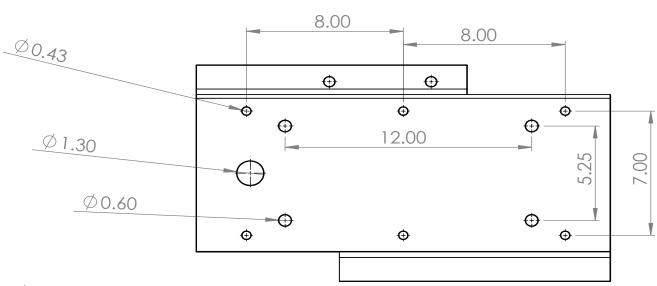
♠ figure 3: Mounting pattern of the PBM1
