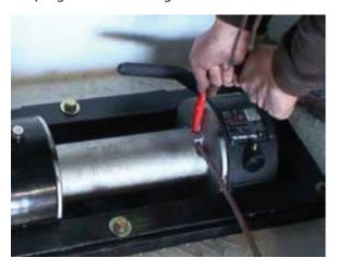
8. Next, power the newly mounted and installed winch. Pull the cable in while applying resistance and tension. Otherwise, the cable will let loose on you and will tangle on the drum.
