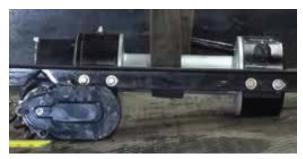
5. Next, connect the power cable from the solenoid to a positive power source. Wire a 4 gauge ground from the winch motor mounting bolt directly to the negative terminal of the truck battery using the PS501 or PS501X2.
